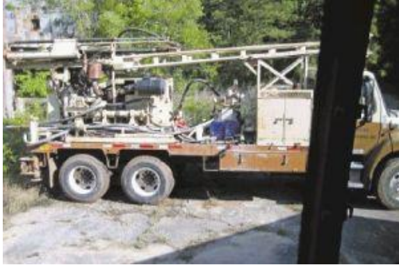
Drill rig for finding chlorinated solvents
